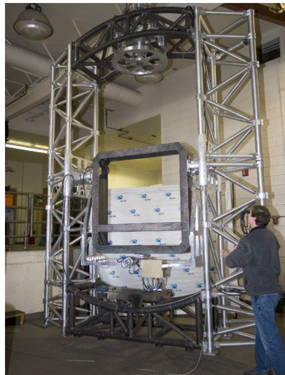
Abb. 30: Die Gondel des SUNRISE-Observatoriums ©High-Altitude Observatory (NCAR, Boulder, Colorado/USA)
